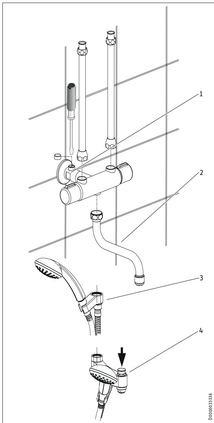
1 Butterfly valve with adjusting screw
